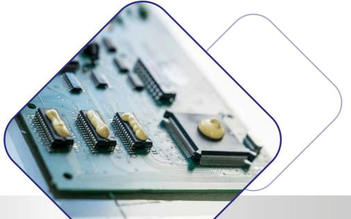
Optimized thermal management for **e-mobility** and performance electronics through - Gap Filler "Liquids".
